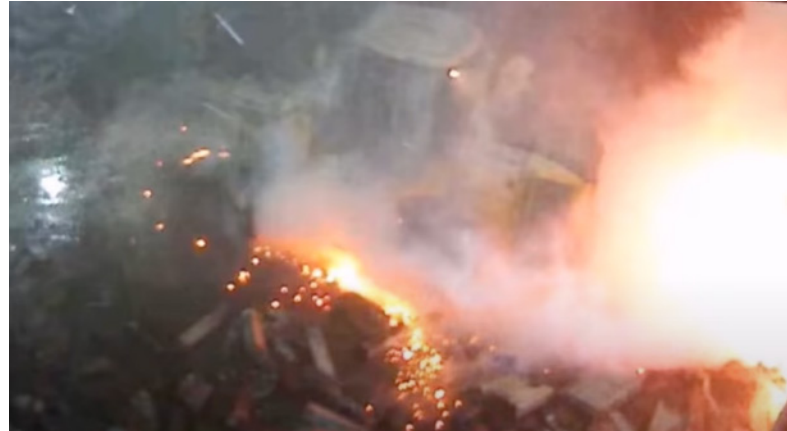
A lithium battery explosion in a lead battery recycling facility.
