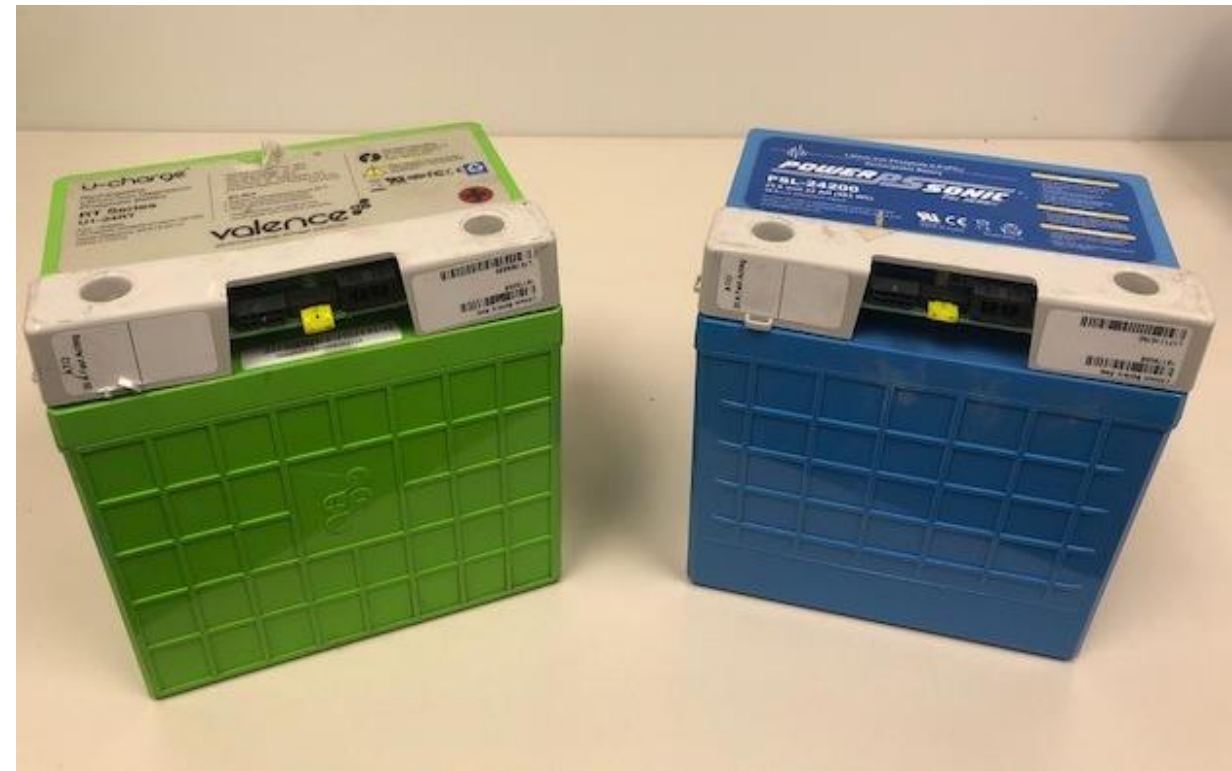
Lithium batteries delivered to Gopher Resources Smelter, Eagan, MN. Discovered inside a lead battery pallet
