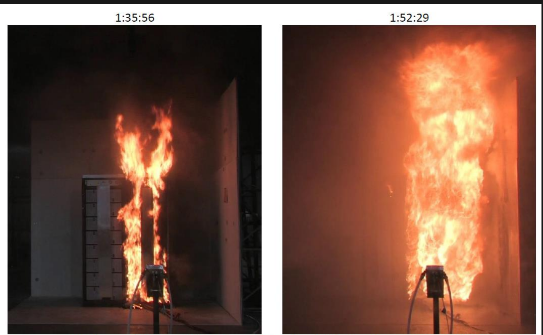
Figure 6-22: Photos of NMC sprinklered test during fire development on main rack: first sprinkler operation (left) and peak heat release rate (right).
